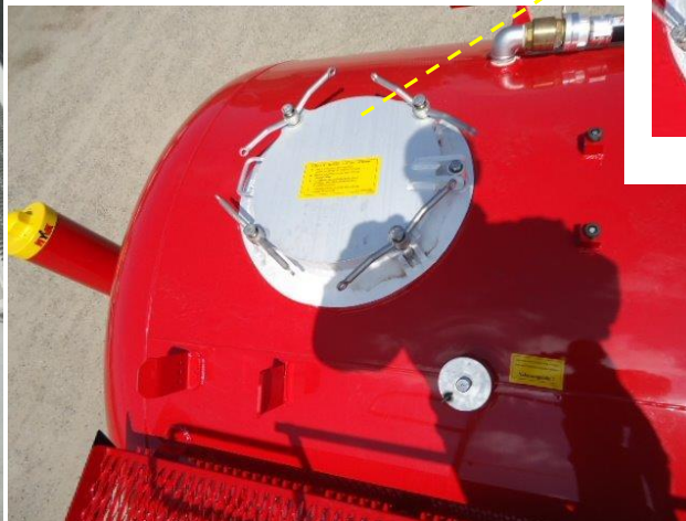
System with 4 bolts and a hinge and safety head.
