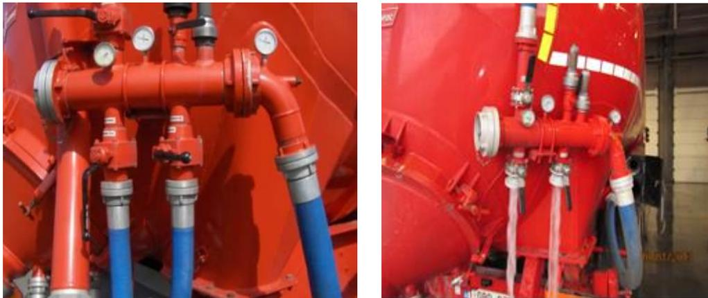
Micro filter is cleaned with air and the internal filter body is cleaned with water
