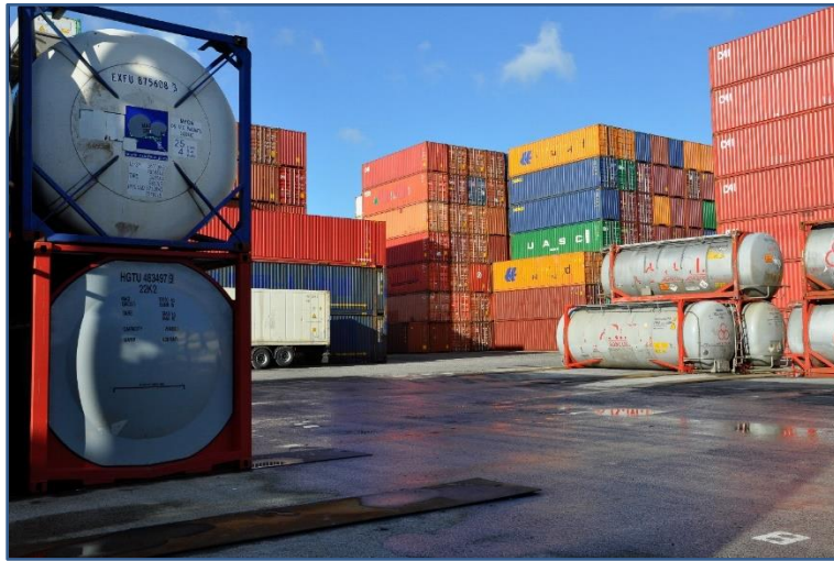
Figure 6 - Stacking of 20'tank containers (left), swap bodies (right) and block stacking of empty box containers (in the back)
