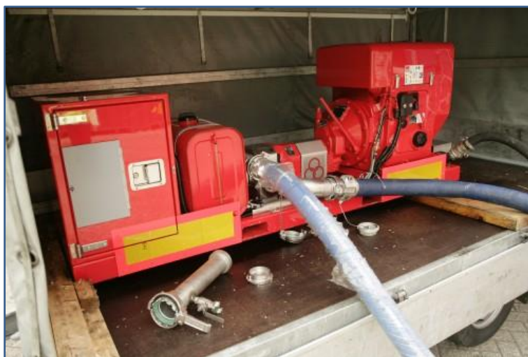
Figure 15 - Pump, running on diesel (no sparks), for chemical liquids
