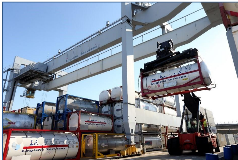
Figure 13 - Rail mounted gantry crane (RMG)
